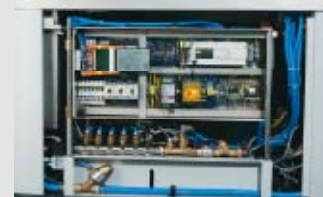
All-in-one and easily accessible: energy source, coolant system, quench system and electrical controls.
