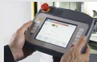
Operating and programming through a touch screen panel.
